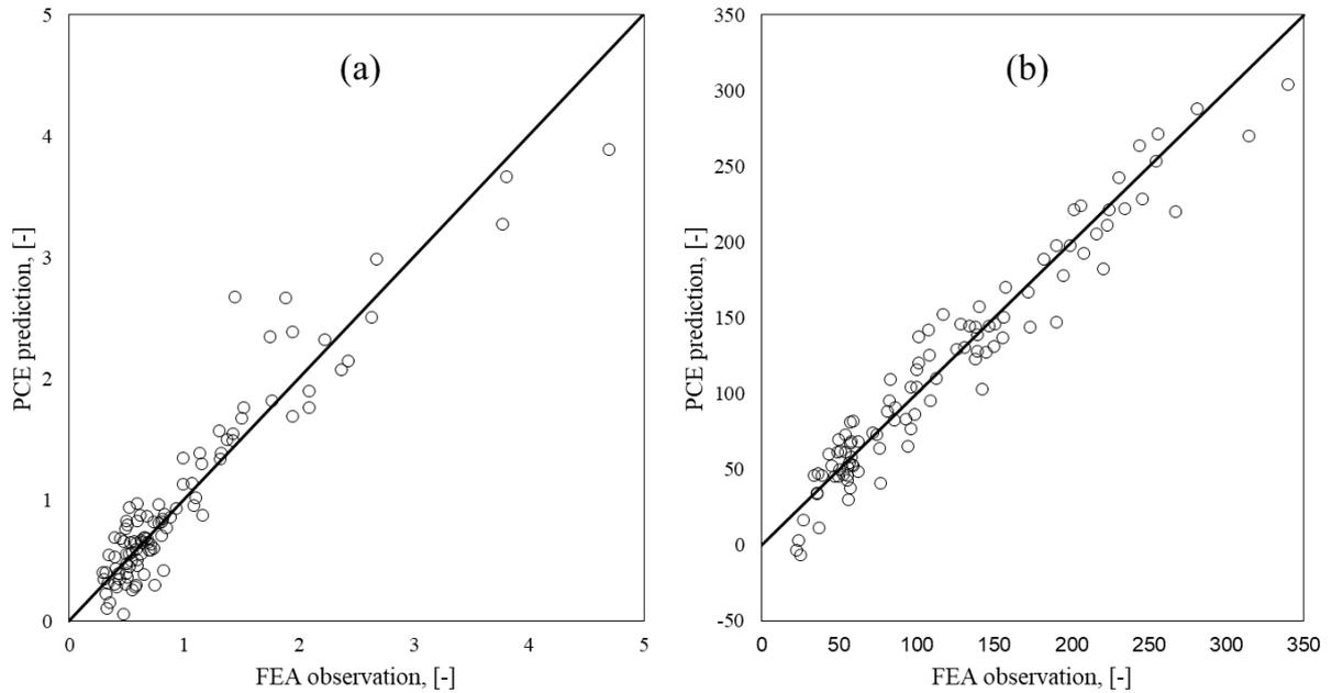
Figure 3. PCE predictions vs FE observations for: (a) normalized ultimate pile capacity,  $\bar{V}$ , and (b) normalized stiffness,  $\bar{K} = \bar{V} / \bar{w}$ , at service load level (50% of  $\bar{V}$ ).
