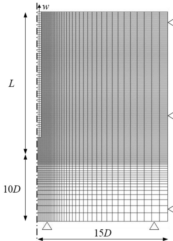
Figure 1. FE model of the anchor pile and boundary conditions.
