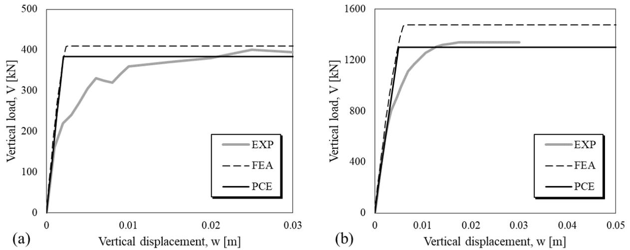
Figure 4. Comparison of PCE and FE evaluations of the experimental load-displacement curves of: (a) Chow (1997) and (b) Rucker et al., (2013).
